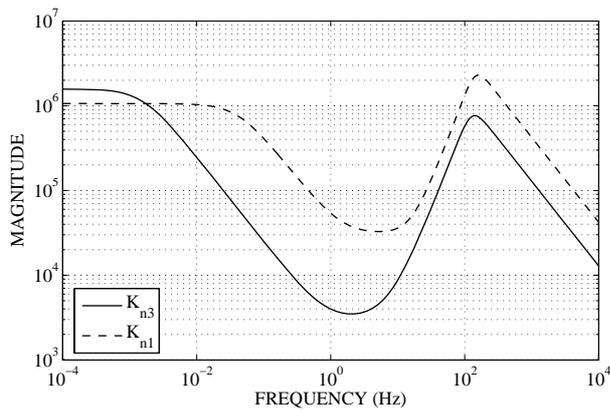
Fig. 1. Frequency Responses of  $\mathcal{H}_\infty$  DIA Controller
