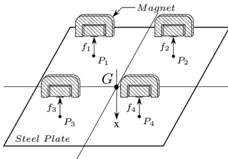
Fig. 3. Magnetically Levitated Steel Plates
