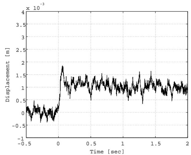
Fig. 9. Step response of *Steel Plate 1* for PID
