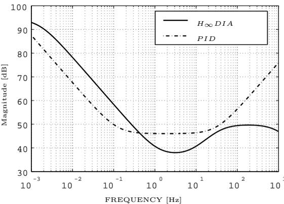
Fig. 4. Frequency Responses of Two Controllers
