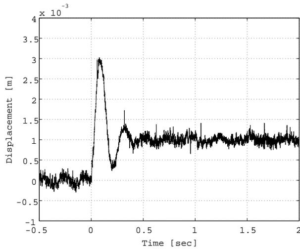
Fig. 6. Step response of *Steel Plate 1* for  $\mathcal{H}_\infty$ DIA
