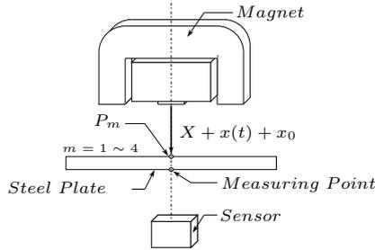
Fig. 2. Position relation between a electro magnet and a sensor
