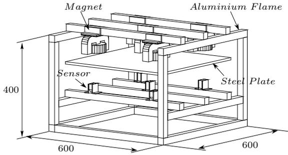
Fig. 1. System structure
