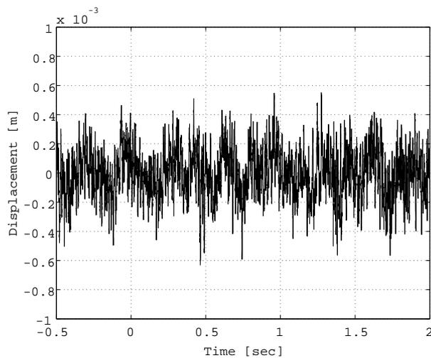
Fig. 7. Steady state of *Steel Plate 2* for  $\mathcal{H}_\infty$ DIA
