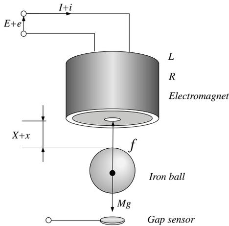
FIGURE 1: Magnetic Suspension System
