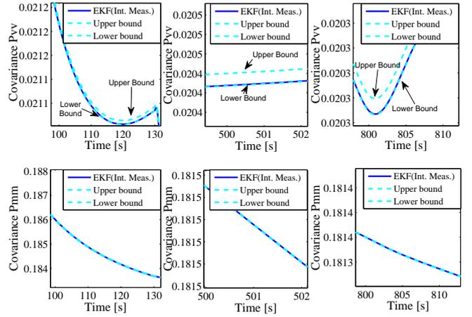
Fig. 5: Upper and lower bound of the estimation for EKF with Intermittent Measurement when measurement data is lost at 100[s], 500[s] and 800[s] for 30[s], 1[s] and 10[s]
