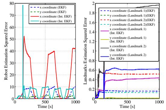
Fig. 6: Performance between EKF and EKF with Intermittent Measurement when measurement data is lost at 100[s], 500[s] and 800[s] for 30[s], 1[s] and 10[s]
