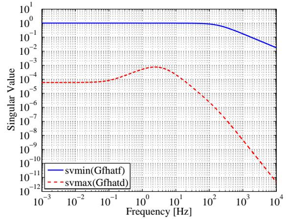
(b) The Singular Value of  $G_{fd}$  and  $G_{ff}$  with Filter B
