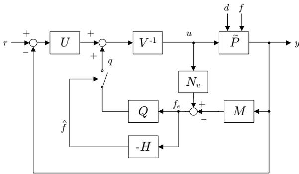
Fig. 6: GIMC-based Fault Tolerant Control
