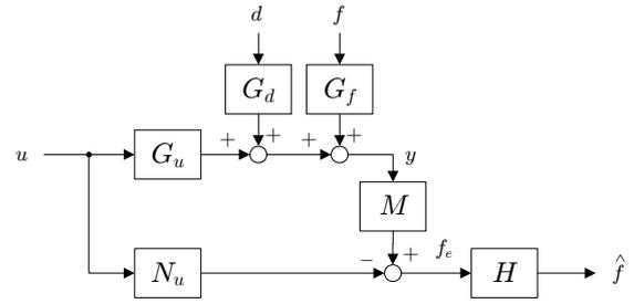
Fig. 1: Block Diagram for the Fault Detection
