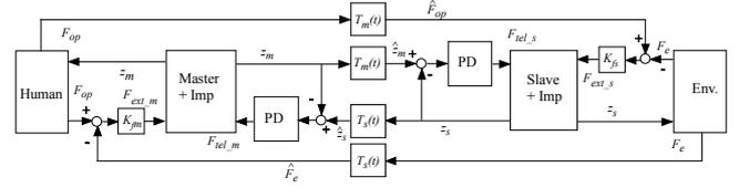
**Figure 2** The master and slave robot dynamics with impedance controller
