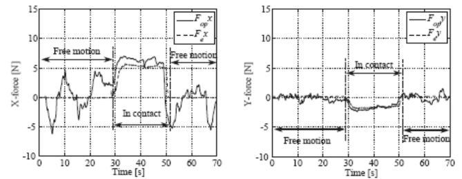
**Figure 10** Varying damping values in contact with environment (Case 2)
