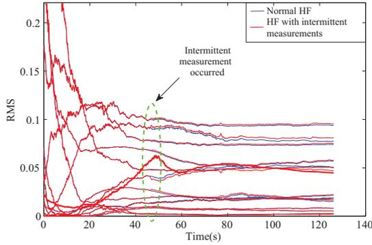
Fig. 3. Some of the estimation errors characteristics when measurements data are missing
