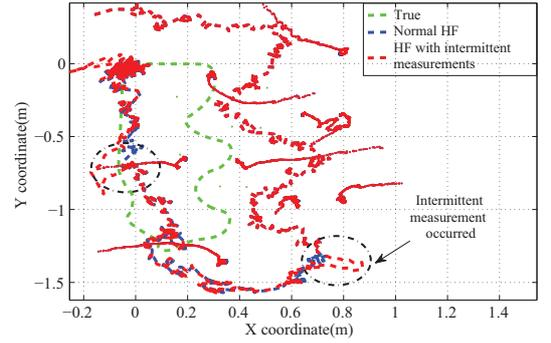
Fig. 2. Map construction between normal HF and HF with partially missing measurement data
