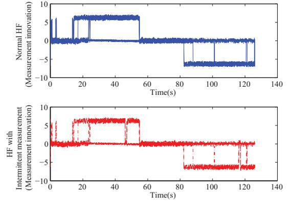
Fig. 5. The measurement innovation characteristics during measurement data loss at the specified time
