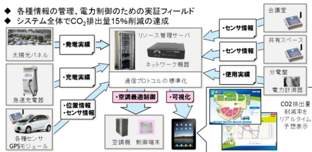
Fig.1 : Field Validation for Energy Management
